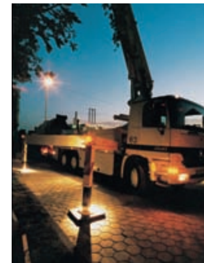
Spotlights facilitate the search for suitable support areas in the dark. Flashlights on the support legs noticeably enhance visibility on the building site.
