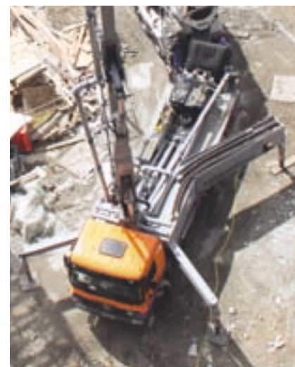
Large storage areas make it possible to carry delivery hoses, delivery pipes and accessories, thereby equipping the M 36-4 for every requirement on the construction site.
