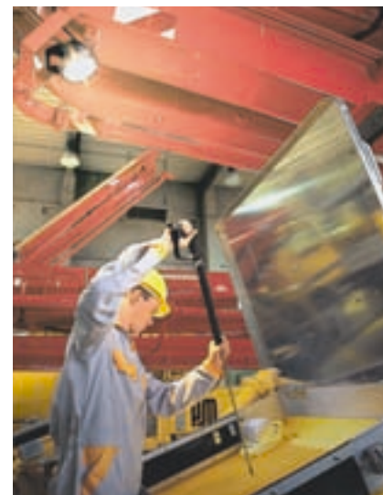
An additional water pump supplies 100 bar high pressure for cleaning work. The hopper is illuminated by a flood light on the boom (Power Plus Kit).
