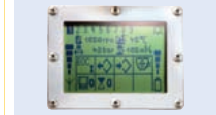
The clear display on the remote control provides up-to-date feedback and system information about the machine. Various parameters can be set here. The strength of the radio signal and charge status of the battery is indicated via bars.
